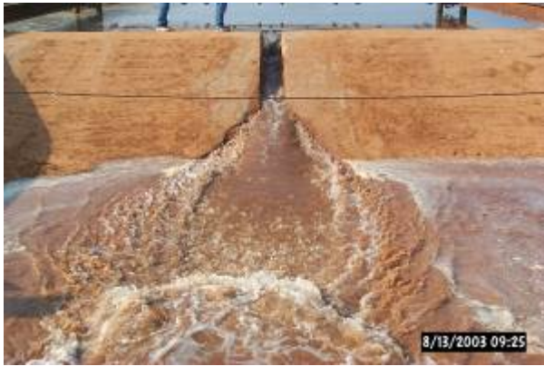
Figure 4. Embankment widening test showing initial notch width.
