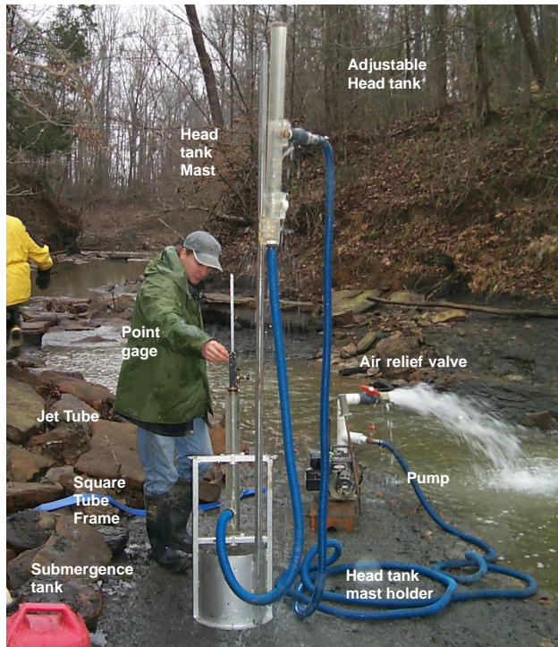
Figure 2. View of apparatus set-up in situ .
