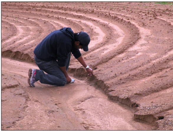
Figure 2. Measuring the depth of ephemeral gullies.
