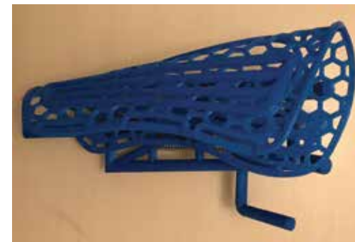
COMPLETED CLASP AND BRACE FOR HOLDING THE SELF-LEVELING SPOON AS DELIVERED TO THE TEAM'S CLIENT IN SPRING 2018
